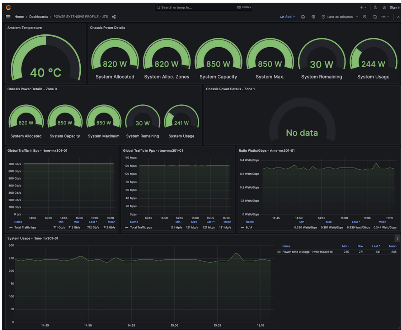
Figure 13: Power Consumption Monitoring
